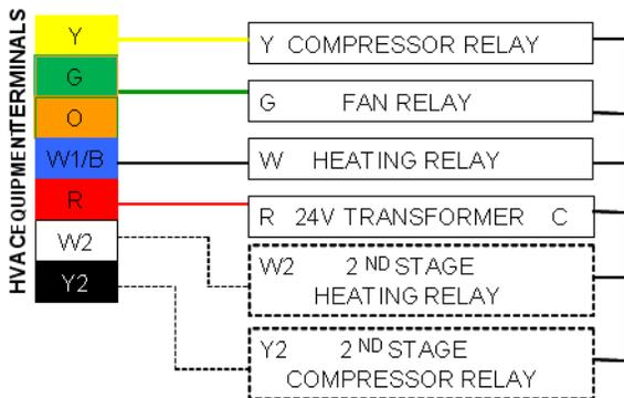
**WIRING DIAGRAM 4 - HVAC Equipment** – Dual Fuel Heat Pump with Fossil Fuel Back-Up
