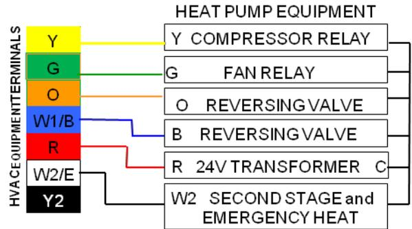
**WIRING DIAGRAM 6** – Two Speed Compressor Heat Pump
